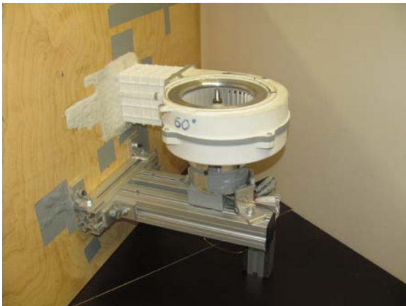
Figure 1: Foto of blower mounted inside the settling box (left), simulation model of settling box with absorbing material and blower geometry (right)
